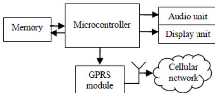
Figure 2. Station Unit Block Diagram
