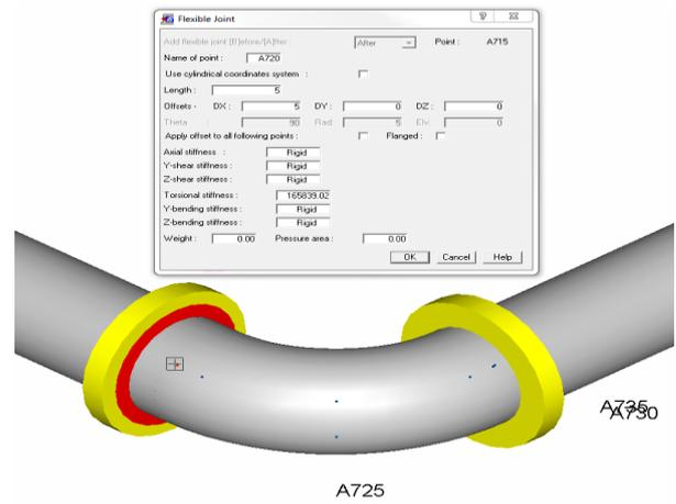
**Figure 6:** Value of torsional stiffness for flexible joints is considered as 165839.02Nm/deg
