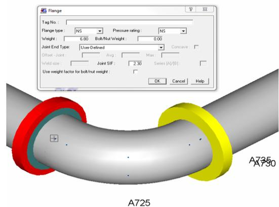
**Figure 4 :** Representation of Grooved coupling for 8” line
