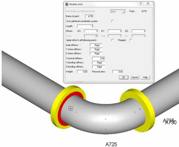
**Figure 5 :** Value of torsional stiffness for flexible joints is considered as 1e-005 Nm/deg
