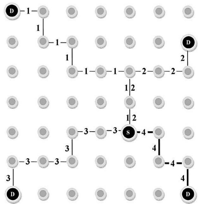
**Figure 3.** Path selection with minimum hop count [5].
