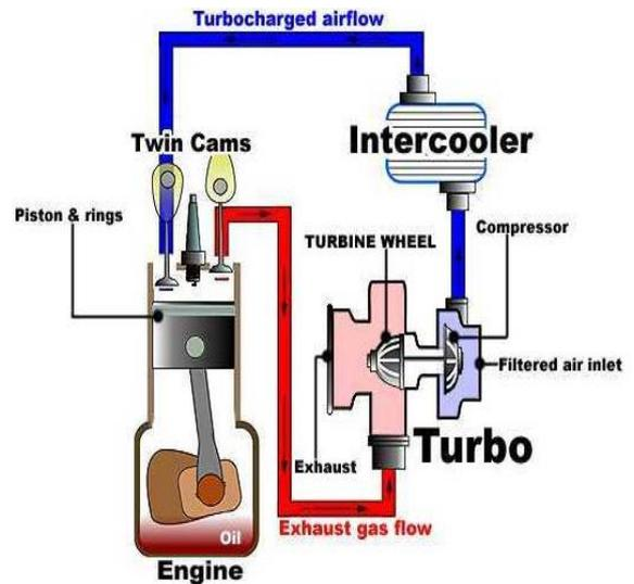
**Figure 2.** Turbocharger working
