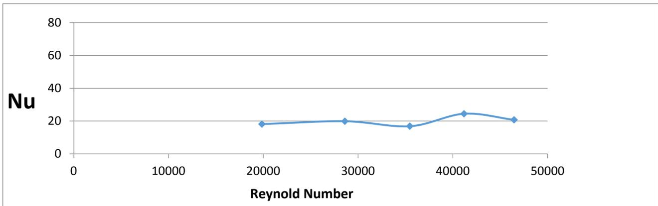
Figure 9. Effects of Reynolds Number on Nusselt Number with Series Connection
