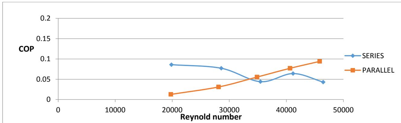
Figure 15. Comparison of COP vs. Reynolds number for both connections
