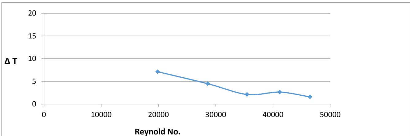
Figure 11. Effects of Reynolds number on temperature distribution with series connection
