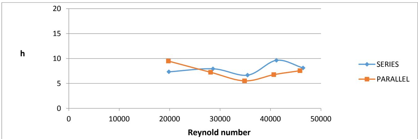
Figure 13. Comparison of heat transfer coefficient vs. Reynolds number for both connection
