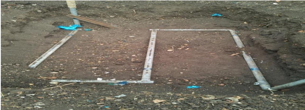
**Figure 5.** Experimental setup in series connection (2.5 inch diameter) without covered soil
