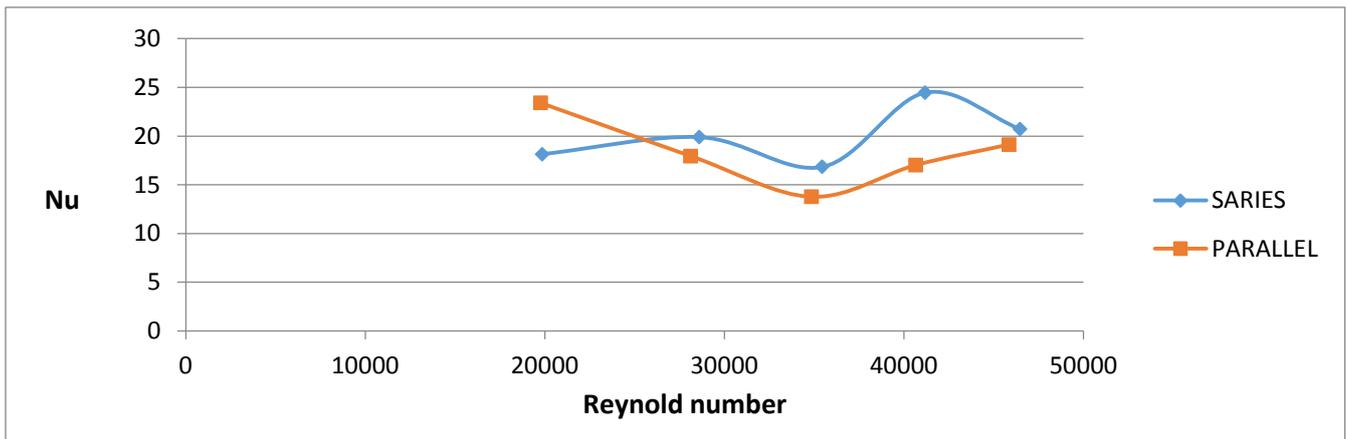
Figure 12. Comparison of Reynolds number vs. Nusselt Number for both connections
