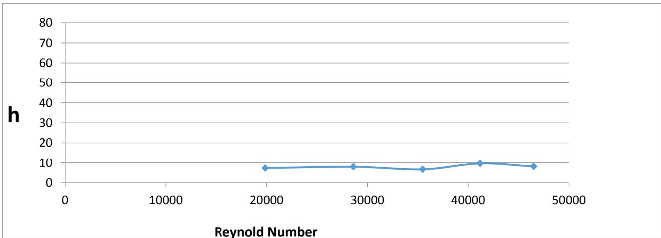
Figure 10. Effects of Reynolds number on Heat transfer Coefficient with series connection
