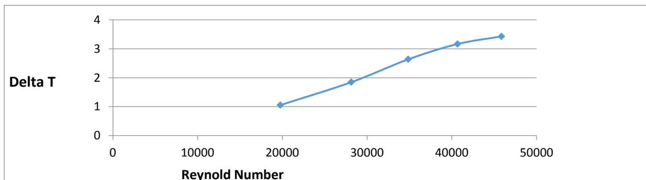
Figure 8. Effect of Reynolds Number on Temperature Difference
