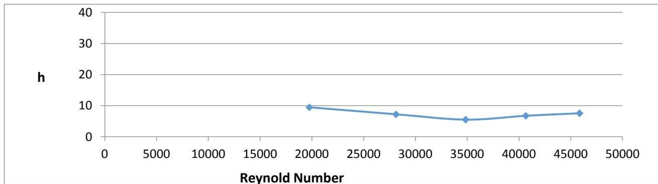
Figure 7. Effect of Reynolds number on Heat transfer Coefficient
