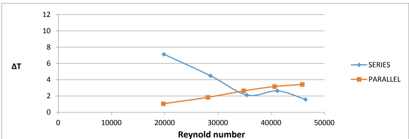
Figure 14. Comparison of temperature difference vs. Reynolds number for both connection
