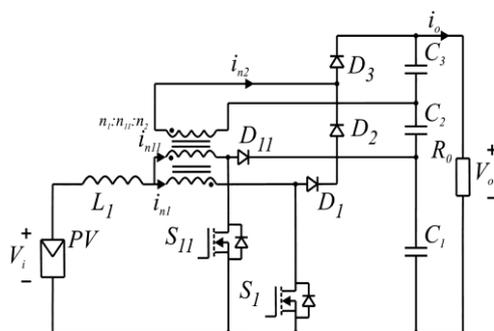
Figure 8. Schematic diagram of push-pull boost converter.
