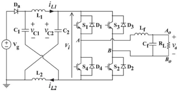
**Figure 4.** Schematic of ZSI
