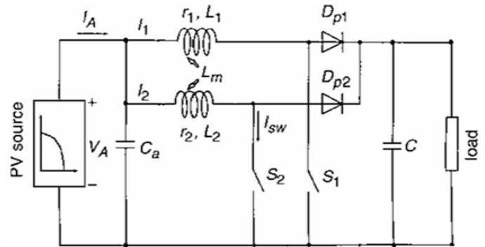
Figure 2. Interleaved boost converter.
