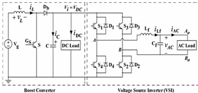
Figure 1. Conventional boost converter.
