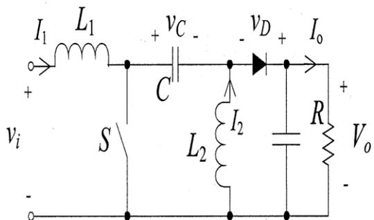
Figure 7. Schematic diagram of SEPIC boost converter
