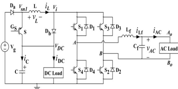
boost the input voltage both the switches in the same leg are turned ON simultaneously.
