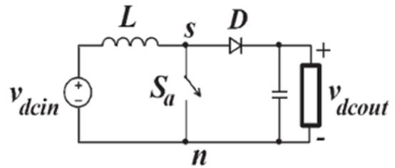
**Figure 10.** Circuit diagram of BDHC converter
