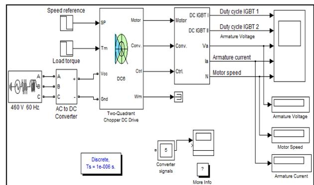
Figure 2. Proposed Model of 2 Quadrant D.C. Drive
