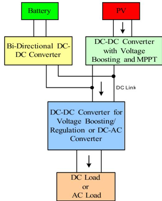
**Figure 9.** Typical Power Conversion Configuration for a Stand-Alone PV System by Das and Agarwal [20]
