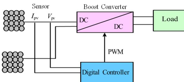
Figure 1. Block Diagram of PV system
