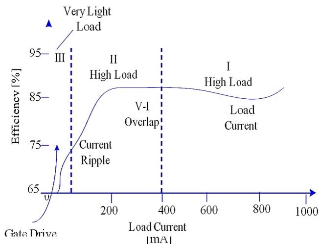
**Figure 4.** DC-DC Converter Efficiency Curve
