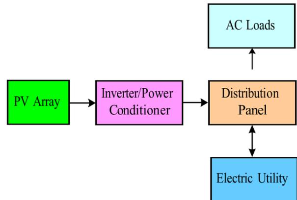
Figure 2. Block Diagram of Grid Interfaced PV System
