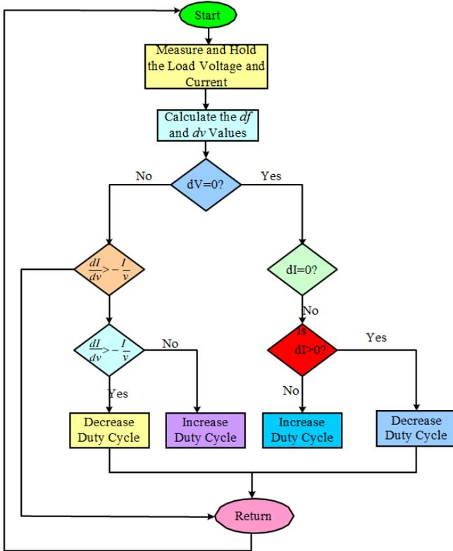
**Figure 6.** Flow Chart of Incremental Conductance
