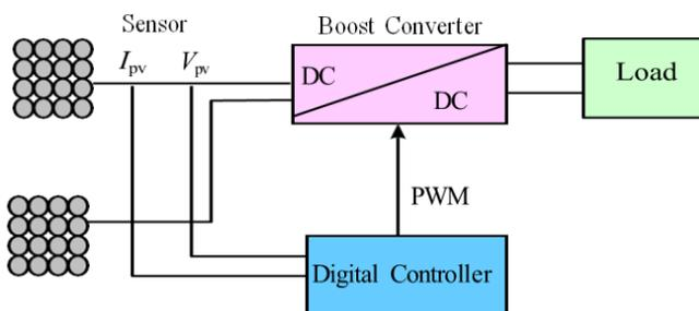
Figure 1. Block Diagram of PV system
