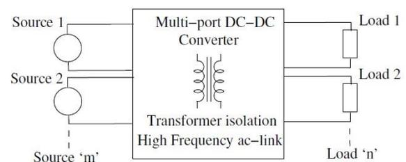
**Figure 1.** Generalized Multiport DC-DC Converter Control of Power Flow between the ports as per application requirement Port voltages can vary widely
