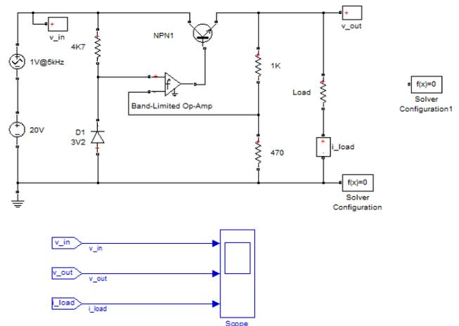
A fluctuating supply is modeled as 20V DC plus a 1V sinusoidal variation. The zener diode D1 sets the non-inverting input of the op-amp to 3.2V, and hence as the op-amp has a large gain, the op-amp inverting input and output are also at 3.2V. Hence the regulator voltage output is regulated to be  $3.2 * (1000 + 470) / 470 = 10V$ .
