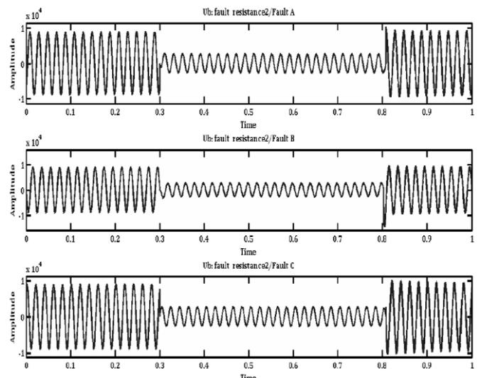
Figure 5: Three Phase Fault Voltage
