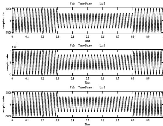
Figure 6: Three Phase Load Voltage before DVR operation
