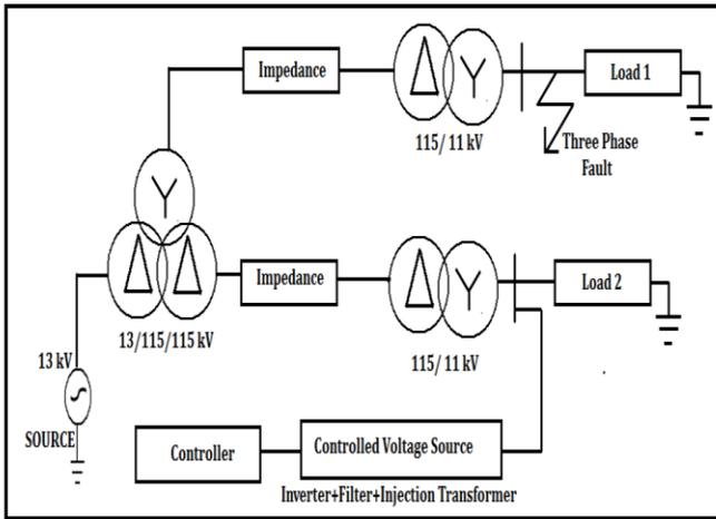
**Figure 1:** Single Line Diagram of the Series Voltage Compensator Test System
