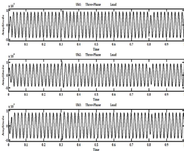
Figure 12: Phase Voltage at Load end after Swell mitigation
