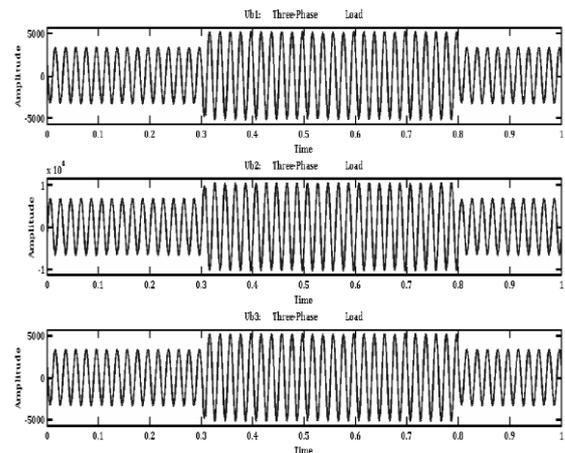
Figure 10: Load Voltage before DVR Operation
