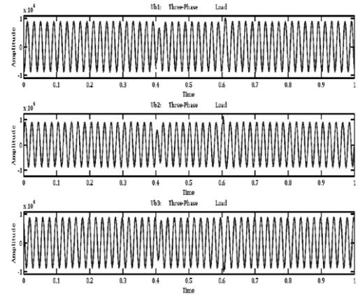
Figure 8: Phase Voltage at Load end after Sag Mitigation
