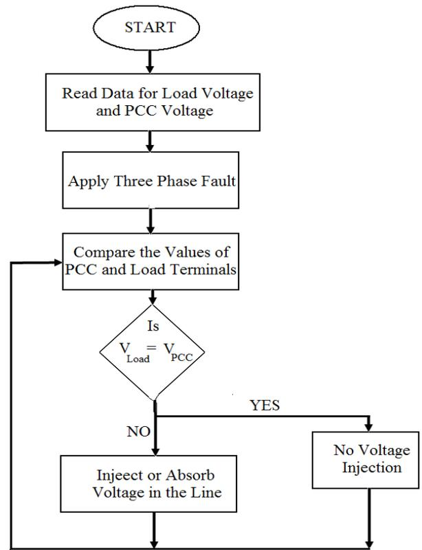
**Figure 2:** Flow Chart for Modelling the DVR test system
