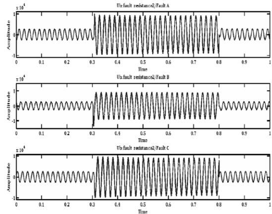
Figure 9: Three Phase Fault Voltages
