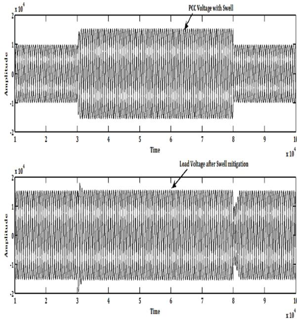
Figure 11: PCC Voltage and Load Voltage after Swell mitigation
