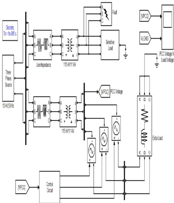
Figure 3: Power Circuit of the DVR Test System
