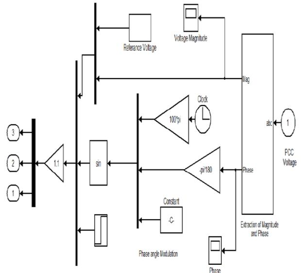
Figure 4: Control Circuit of the DVR Test System
