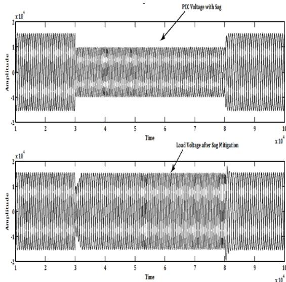
Figure 7: PCC Voltage and Load Voltage after Sag Mitigation
