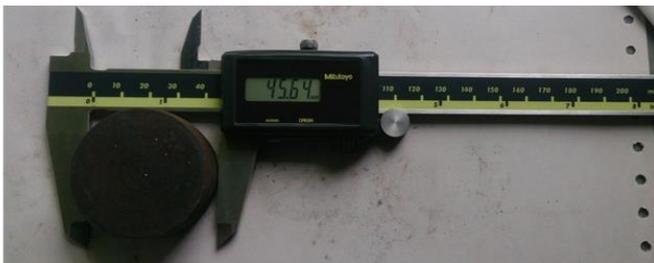
**Figure 6 :** Measurement of dimensions of billet after compression
