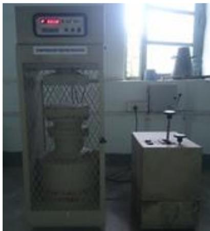
**Figure 2 :** Compression Testing Machine
