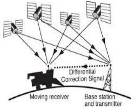
**Figure 2 : Real-time differential GPS**
