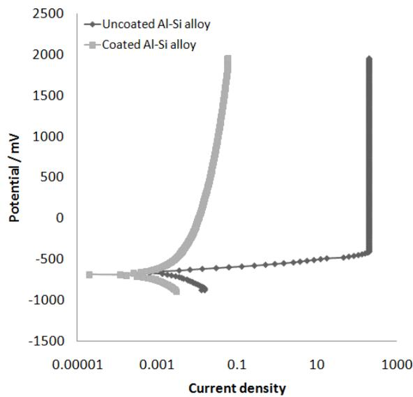
**Fig. (4):** Polarization curves of uncoated and coated Al-Si alloy by  $\text{Al}_2\text{O}_3/\text{SiC}/\text{ZrO}_2$  nanoparticles in 3.5% NaCl solution.
