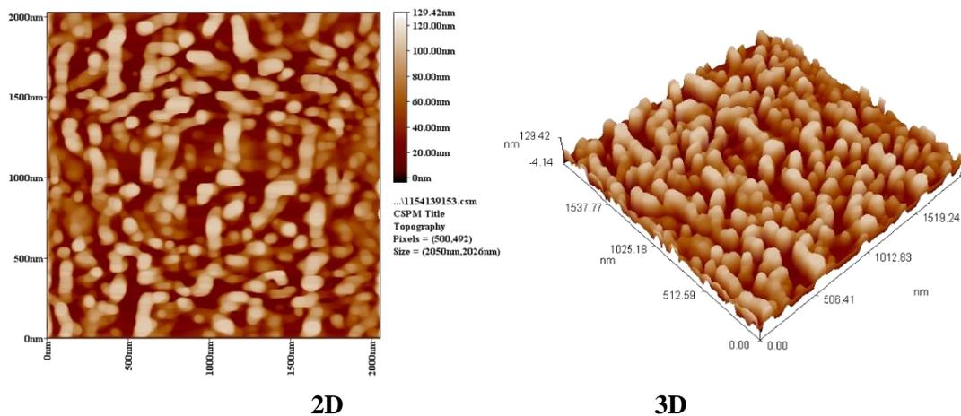
**Fig. (1):** AFM images of coated Al-Si alloy by nanoparticles.
