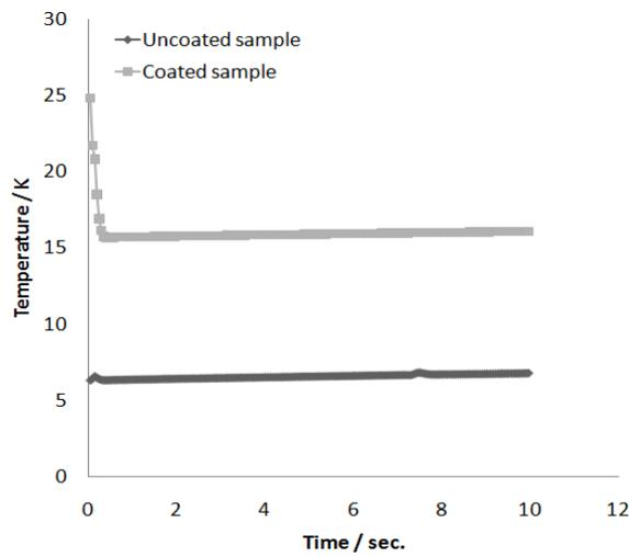
**Fig. (3):** Temp. – time relationship for uncoated and coated Al-12Si alloy
