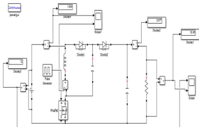
Figure 9 : Simulink Model for Luo converter
