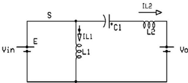
Fig 2: Luo converter with MOSFET ON condition
