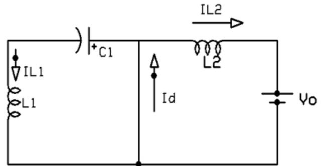
Fig 3: Luo converter with MOSFET OFF condition
