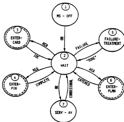
**Figure 6:** Mealy-Graph for the MS access procedure.
