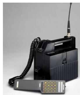
**Figure 5:** Transportable mobile station.
