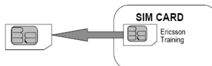
Figure 12: Plug-in SIM card [9].
