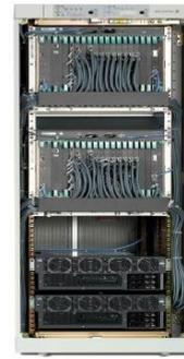
**Figure 17:** Base Station Controller
