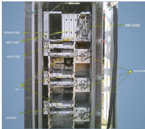
**Figure 16:** Architecture of Base Transceiver Station [22].
