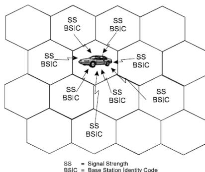
Figure 8: Monitoring Broadcast Control Channel carriers.
