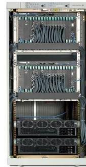
**Figure 17:** Base Station Controller
