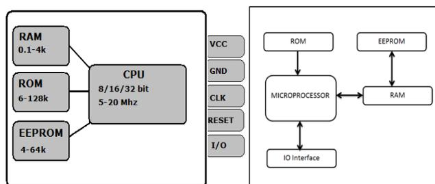
Figure 10: SIM Card structure [17].
