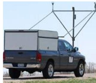
**Figure 3:** Vehicle-mounted mobile station.
