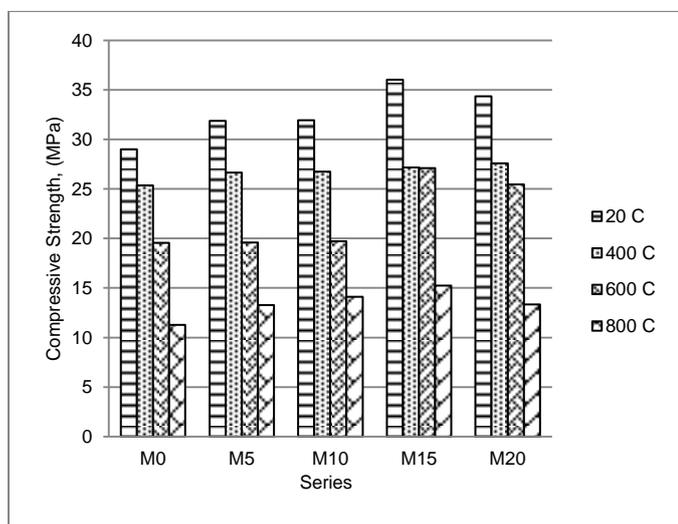
**Figure 3.** Relationship of Temperatures-Compressive Strength Series
