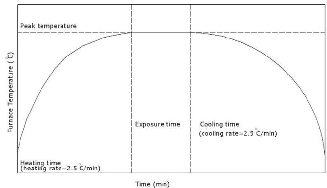
**Figure 2.** Temperature-time curve heating, exposure, cooling
