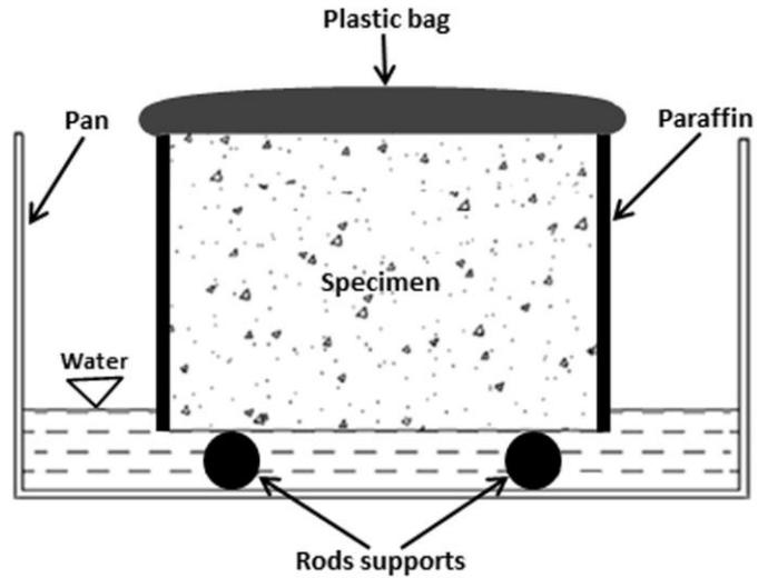
**Figure 1.** Experimental setup for sorptivity test [12]
