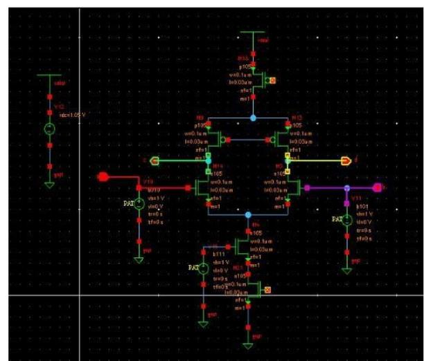
**Figure 3 :** Design of Current Mirror Sense Amplifier using MTCMOS technique under 30nm technology.
