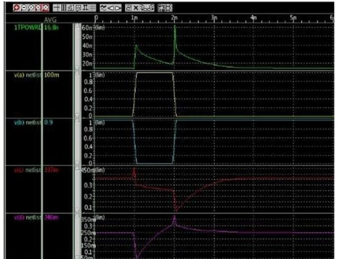
**Figure 7:** Output waveform of the current mirror sense amplifier (MTCMOS) with supply voltage 5V.
