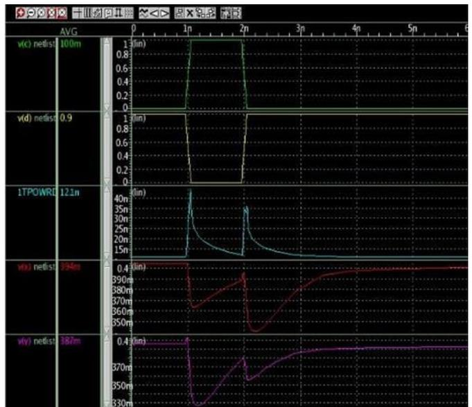
**Figure 8 :** Output waveform of the PROPOSED SYSTEM (conventional voltage latch sense amplifier-MTCMOS) with supply voltage 5V
