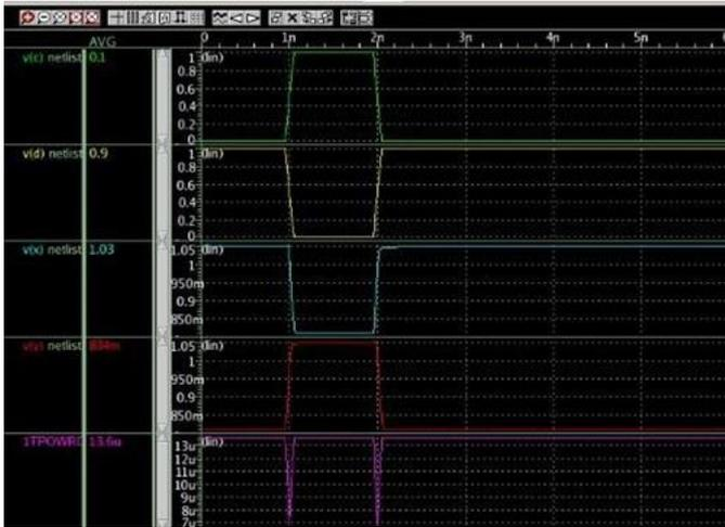
**Figure 5:** Output waveform of the conventional voltage latch sense amplifier with supply voltage 5V
