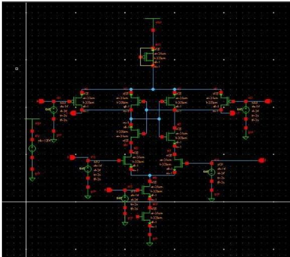
**Figure 4 :** Design of Conventional Voltage Latch Sense amplifier Using MTCMOS technique Under 30nm Technology.
