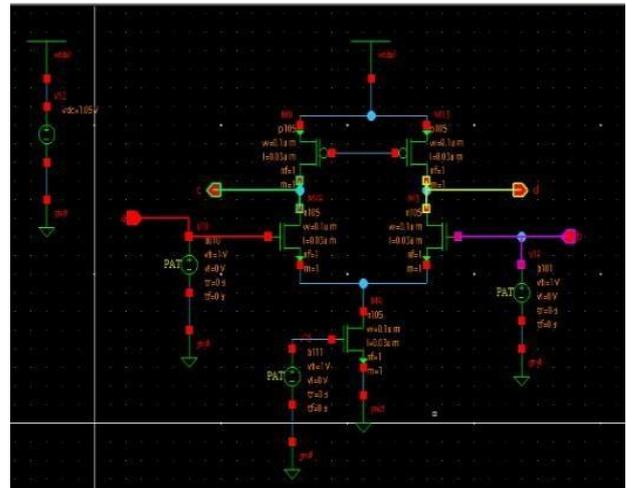
**Figure 2 :** Design of Current Mirror Sense Amplifier under 30nm technology.
