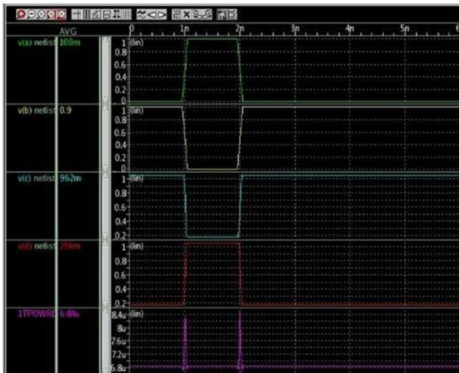
**Figure 6:** Output waveform of the current mirror sense amplifier with supply voltage 5V
