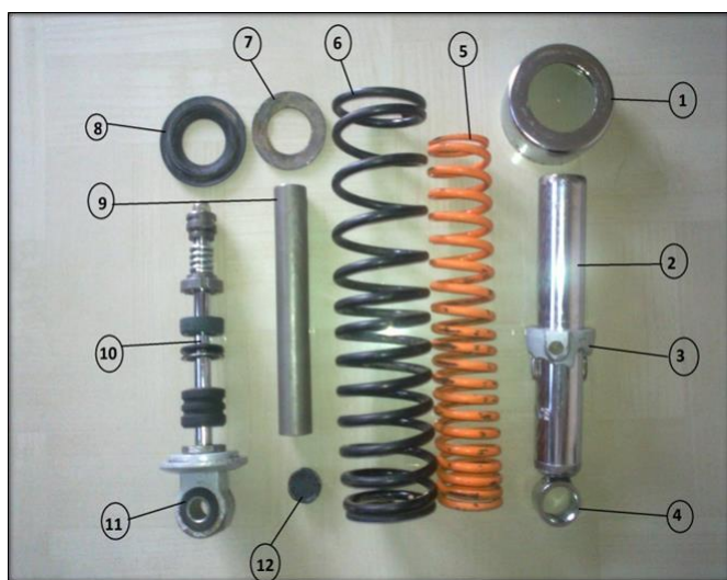
Figure 2. Elements of Twin tube rear shock absorber
