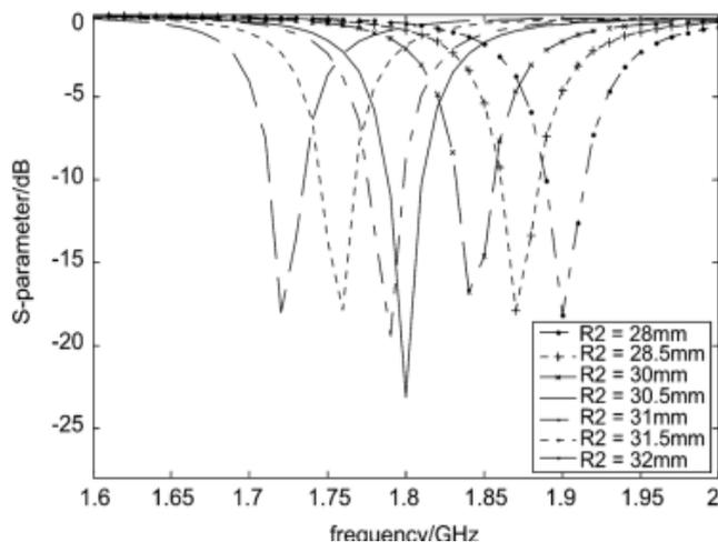
**Figure 10.** Simulated  $S_{11}$  with different  $R_2$  for Narrow Half-Ring and Half-Circular Patch
