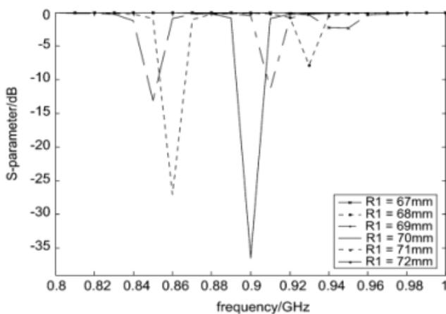
**Figure 9.** Simulated  $S_{11}$  with different  $R_1$  for Narrow Half-Ring and Half-Circular Patch
