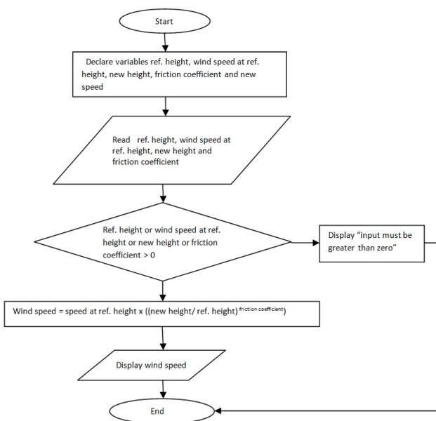
**Figure 1:** flow chart for computing wind speed at varying heights
