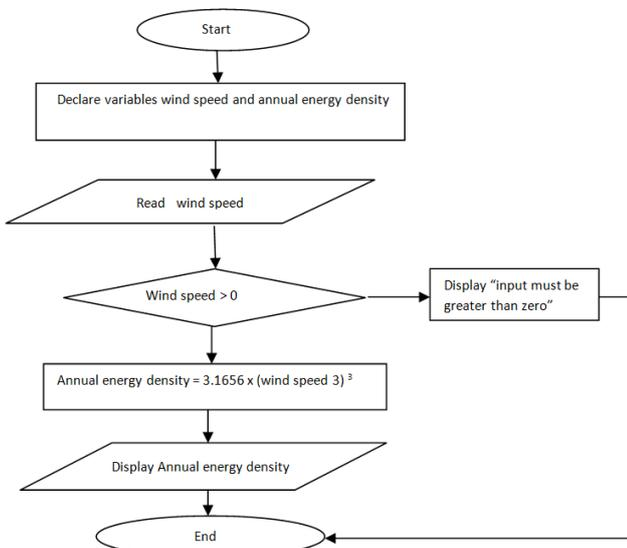
**Figure 2 :** Flow chart for computing annual wind electric energy density.
