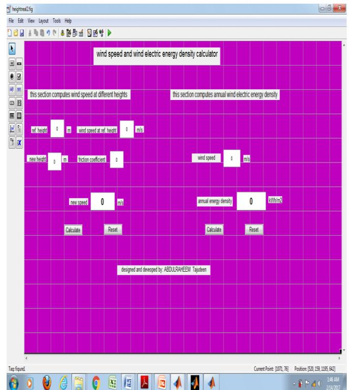
**Figure 3.** Developed graphical user interface for wind speed and wind electric energy density computation.
