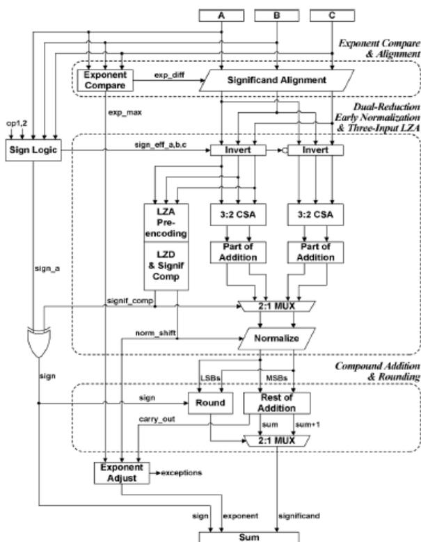
Figure 1. Existing fused floating point three term adder
