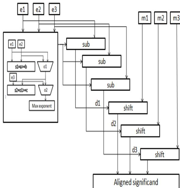
**Figure 3.** Proposed Exponent comparison and significand alignment block
