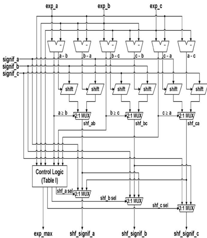
**Figure 2.** Existing Exponent comparison and significand alignment block
