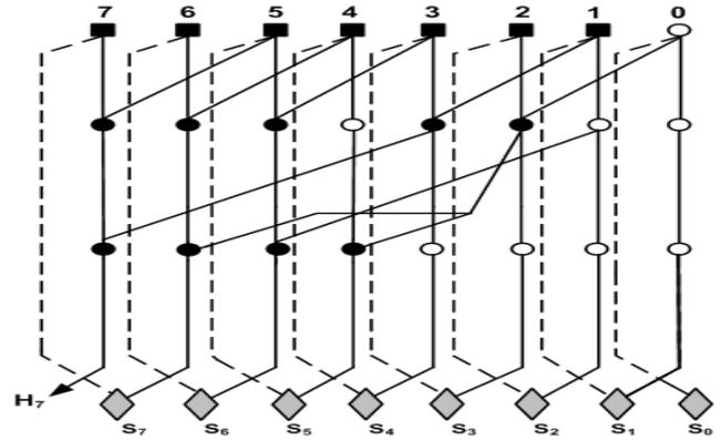
Figure 4. Ling adder for mantissa addition
