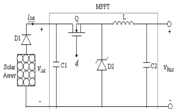
Figure 2. Circuit schematic of the photovoltaic power subsystem
