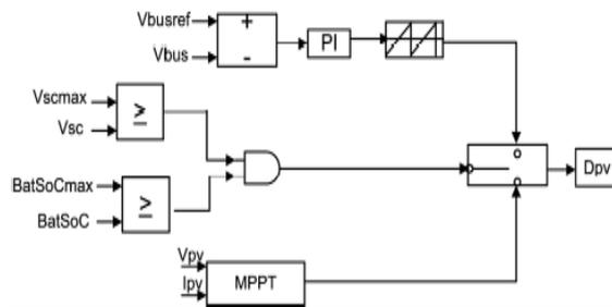
**Fig. 4.** Modeling of PV controller
