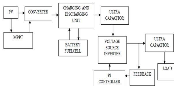
Figure 1. PV-FC-battery-SC hybrid system
