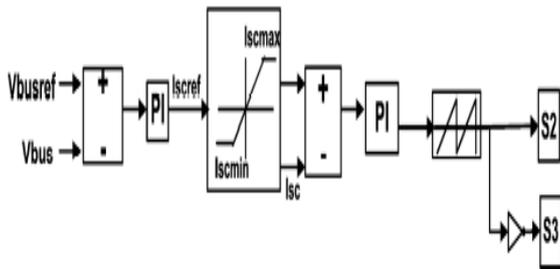
Fig. 5. Modeling of SC Controller
