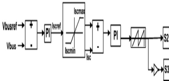
Fig. 5. Modeling of SC Controller
