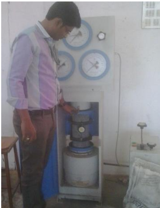
Figure 8. Cylinder fitted with Compressometer and tested in UTM 0.5% Plastic Straws
