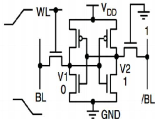
**Figure 3.** Adiabatic 6 Transistor SRAM Structure
