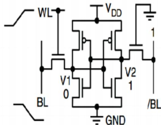
**Figure 3.** Adiabatic 6 Transistor SRAM Structure
