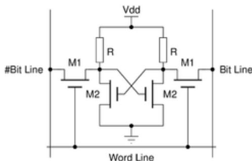
**Figure 2.** 4-T SRAM Cell
