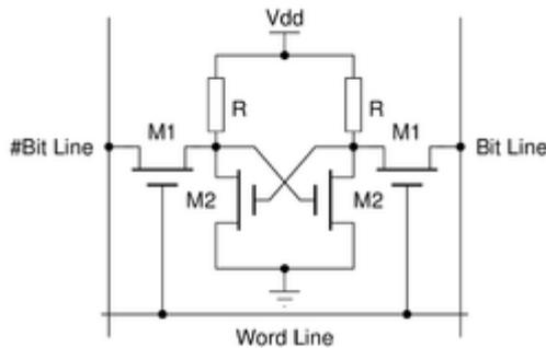
**Figure 2.** 4-T SRAM Cell
