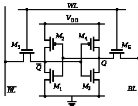
Figure 1. Structure of 6-T SRAM Cell
