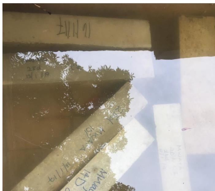
Figure 4 : Beams, cubes and cylinders curing
