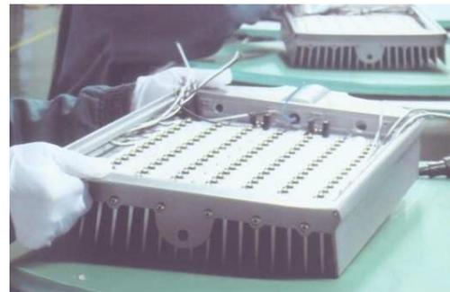
**Figure 1.** The heat sink of LED street lamp
