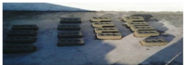
Figure 2. Casting of papercrete bricks
