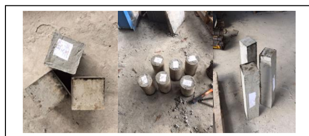
Figure 6. Specimen after removing molds
