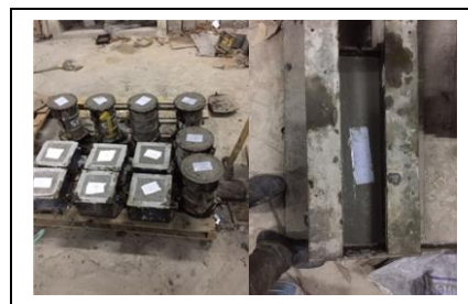
Figure 5. Casting of cubes, cylinder and beams
