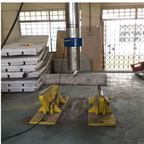
Figure 12. Determination of flexural strength
