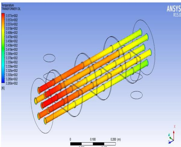
Figure 3. Temperature distribution for the Transformer oil
