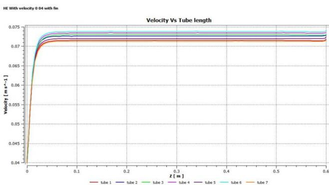
Figure 9. HE with velocity of 0.04m/s with fin
