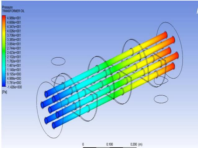
Figure 1. Pressure distribution for the transformer oil
