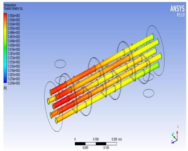
Figure 6. Temperature distribution for the Transformer oil
