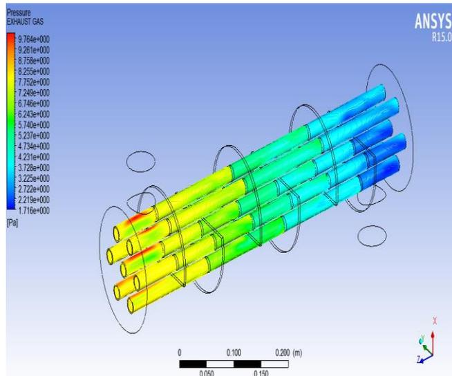
Figure 7. Pressure distribution for the Exhaust gas
