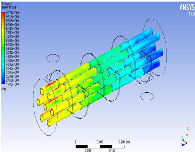
Figure 2. Pressure distribution for the Exhaust gas
