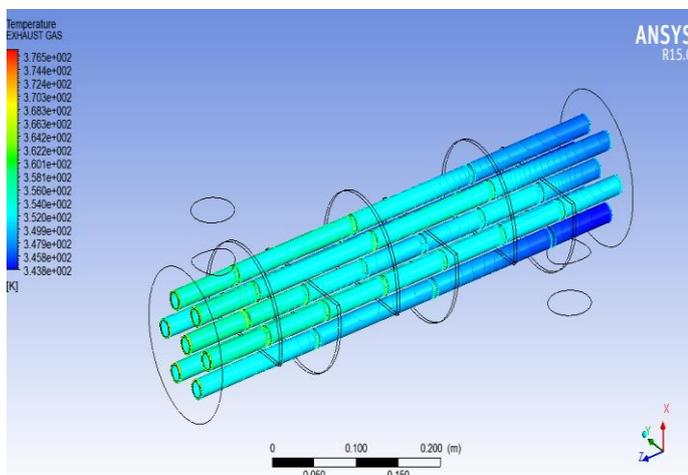
Figure 8. Temperature distribution for the Exhaust gas
