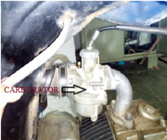
Figure 6. Modification of carburetor
