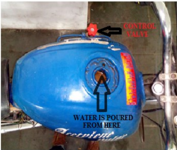
Figure 2. Designation of Tank where water to be poured.
