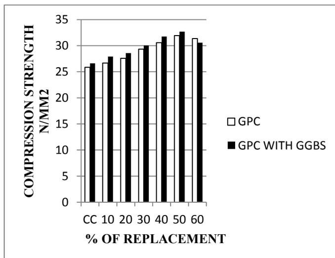
**Figure 2.** Average Compressive strength for all replacement IN CURING after 7days.
