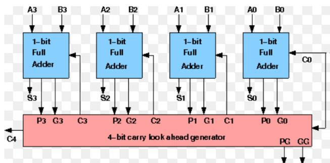
**Figure 1.** Block diagram of carry look ahead adder
