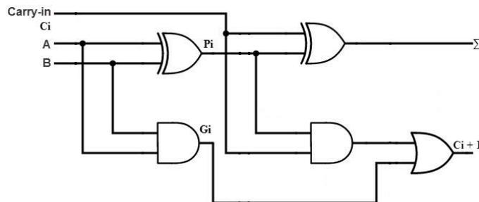
**Figure 2.** Circuit diagram of carry look ahead adder
