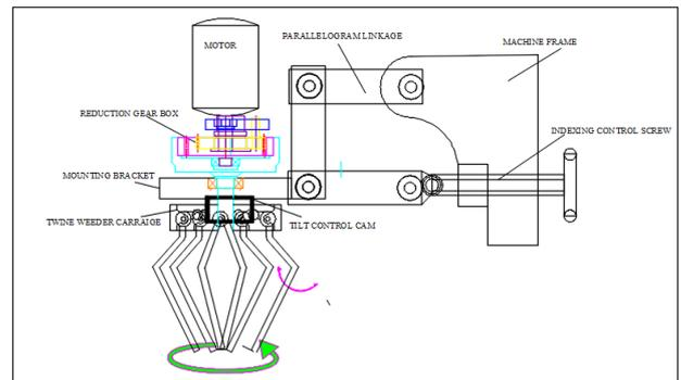
Figure 1. Design of the Kinematic linkage for weeder
