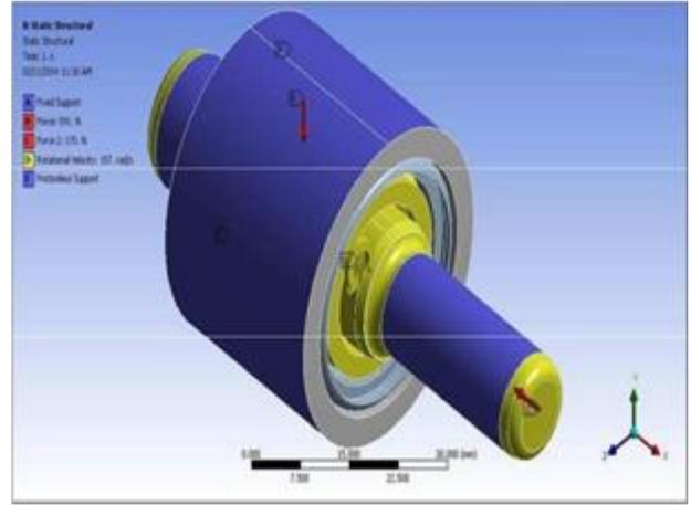
Figure 5. Loading and Boundary Conditions
