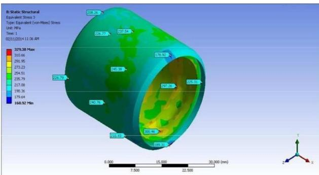
Figure 16. Equivalent Stresses for Sleeve
