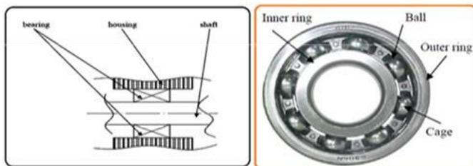
**Figure1.** Rolling Bearing
