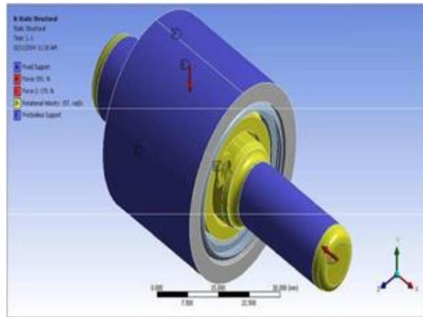
Figure 5. Loading and Boundary Conditions
