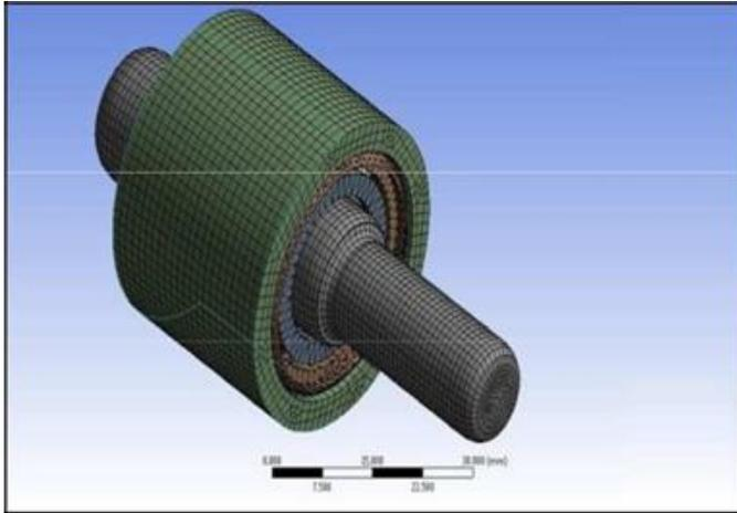
Figure 3. Mesh Generation of Whole Assembly
