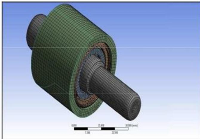
Figure 3. Mesh Generation of Whole Assembly
