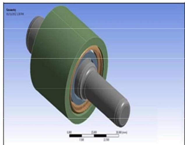
Figure 2. Integral Shaft Bearing
