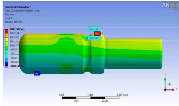
Figure 11. Deformations for Shaft (Y-Direction)
