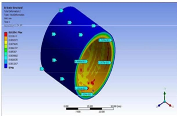
Figure 9. Total Deformation for housing
