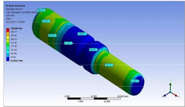
Figure 10. Equivalent Stresses for Shaft
