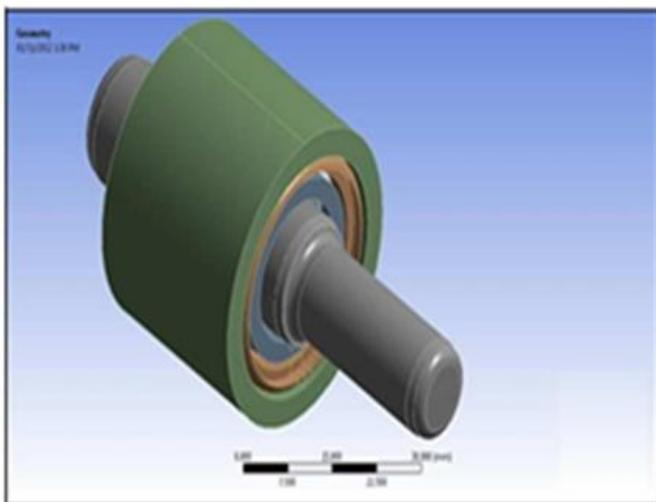
Figure 4. Integral Shaft Bearing
