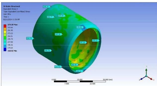
Figure 16. Equivalent Stresses for Sleeve
