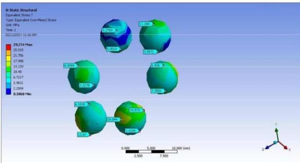
Figure 14. Equivalent Stresses for Ball
