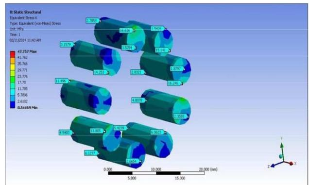
Figure 12. Equivalent Stresses for Rollers
