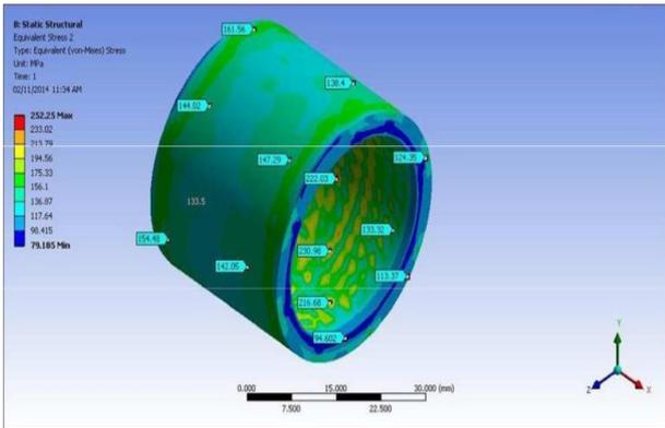
Figure 8. Equivalent Stress for housing
