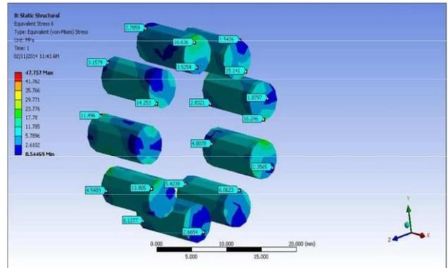
Figure 12. Equivalent Stresses for Rollers
