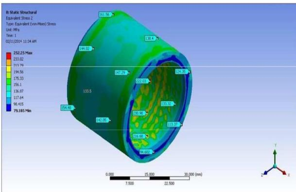
Figure 8. Equivalent Stress for housing
