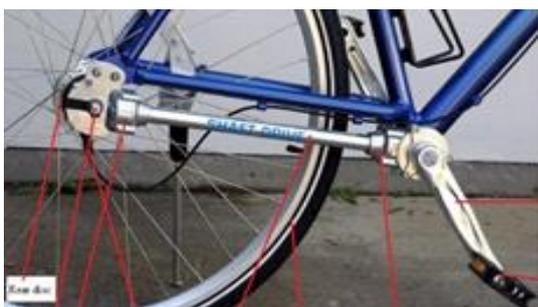
**Figure 3.** Components of shaft driven bicycle
