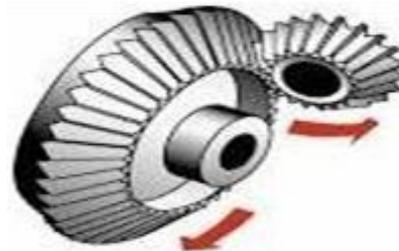
Figure 4. Bevel Gear
