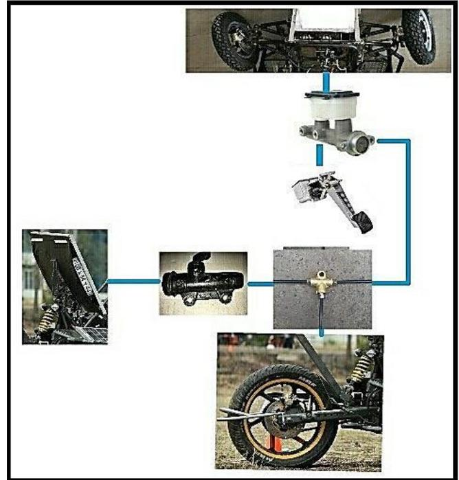
**Figure 2:** Circuit Diagram of Hydraulic Disc Brake System
