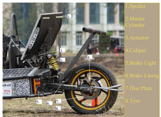
**Figure 3 :** Components of Disc Brake System
