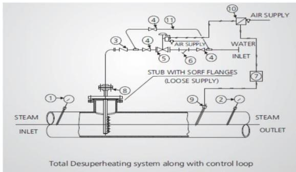
Figure 4 : Total de-superheating system along with control loop
