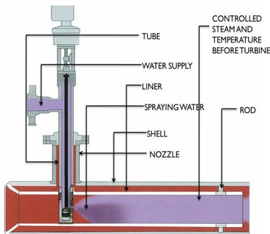
**Figure 1:** Venturi type de-superheater
