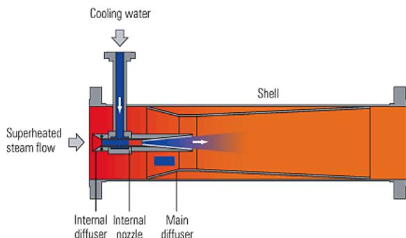
Figure 2: Working of venturi type de-superheater
