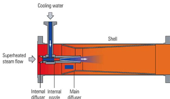
Figure 2: Working of venturi type de-superheater
