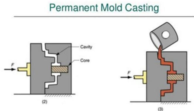
Steps in permanent mold casting: (2) cores (if used) are inserted and mold is closed, (3) molten metal is poured into the mold, where it solidifies.
