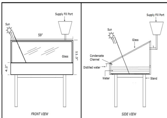
Figure 2.1: Schematic Diagram of Solar Still
