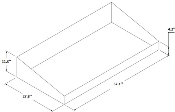
Figure 2.3: CAD model Inner Blackened Tray
