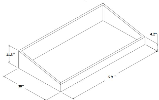
Figure 2.2: CAD model Outer Frame
