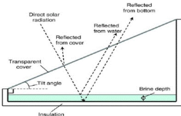
**Figure 1.1:** Solar Still Diagram
