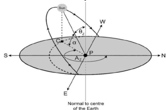
Figure 1.2: Zenith angle ( $\Theta_z$ ), the altitude angle ( $\alpha$ ), and the Azimuth Angle ( $Az$ ) of the Sun when view from point P on the Earth's surface.
