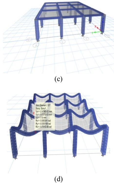
**Figure 2 :** a) Flat slab building before analysis. b) Flat slab building after analysis. c) conventional slab building before analysis. d) conventional slab building after analysis.
