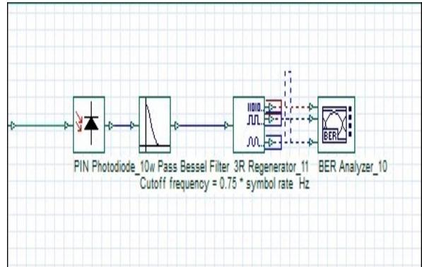
Figure 7: Subsystem-3 (Receiver Section)
