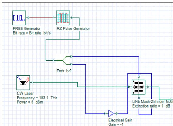
Figure 6: Subsystem-2 (Transmitter Section)
