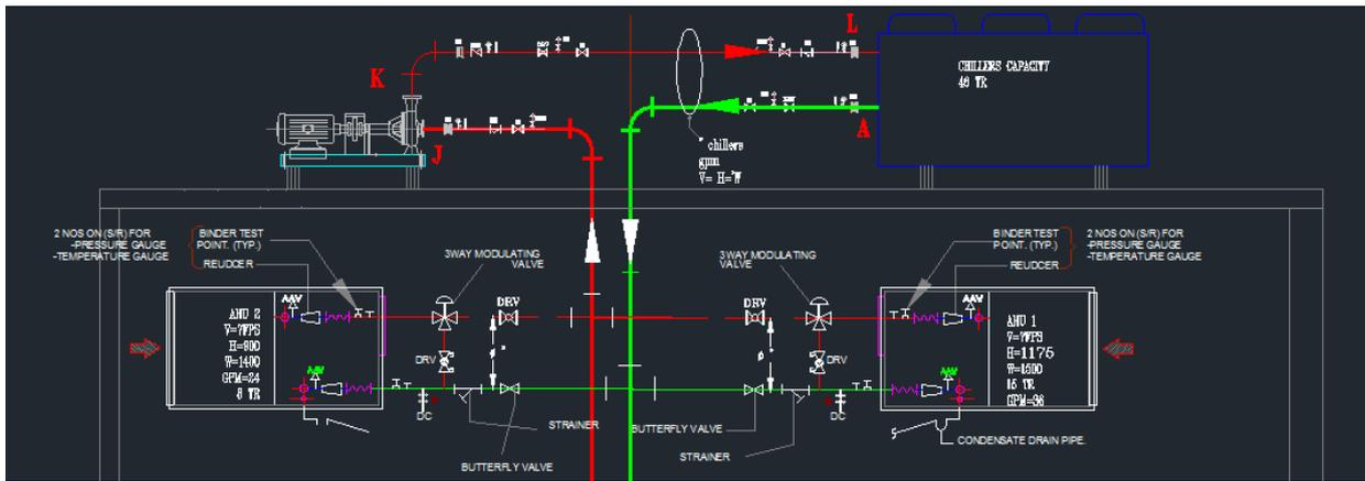
**Figure 3.** Chilled water piping routing and chilled water pump
