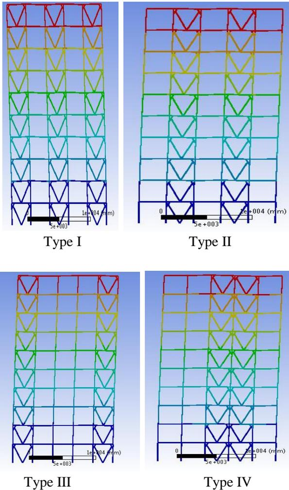
**Fig.3** Models after deformation for Chevron knee braced frame.
