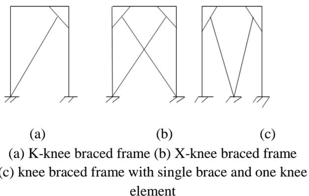
**Figure 1.** Types of knee brace frames
