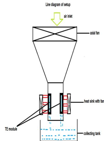
Figure 2. Line diagram of experimental Setup
