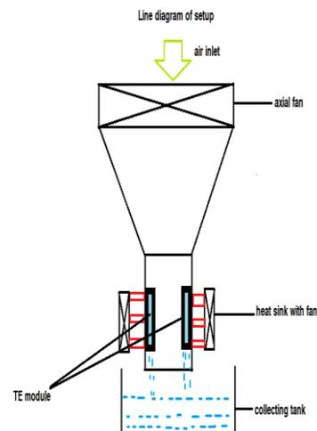
Figure 2. Line diagram of experimental Setup
