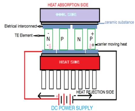
Figure 1. Thermo Electric Module
