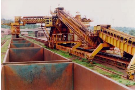
Figure 1. Typical Mobile fixed chute Wagon Loader
