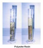
**Figure 3.** Density and volume measurement of fiber and FRP
