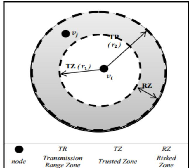
**Figure 3.** Transmission range zones <sup>[6]</sup>
