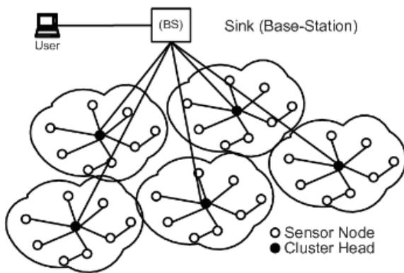
**Figure 2.** General Architecture of sensor network <sup>[6]</sup>
