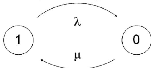
**Figure 3:** State Transition diagram for two state random jammer
