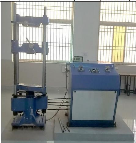
Figure 1: Experimental setup of tensile test
