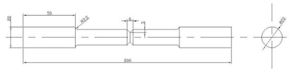
Figure 3: Specimen with V2 Notch
