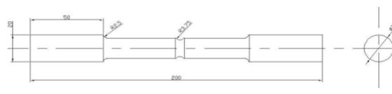
Figure 4: Specimen with U1 Notch
