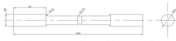
Figure 4: Specimen with U1 Notch
