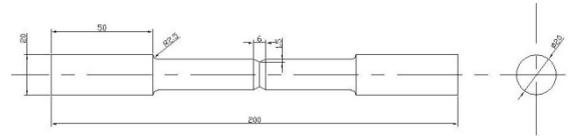
Figure 2: Specimen with V1 Notch
