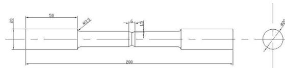
Figure 2: Specimen with V1 Notch
