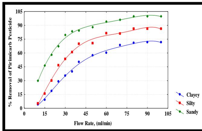
**Figure 8:** Effect of flow rate on the % removal of pirimicarb pesticide from three different types of Iraqi soils using distilled washing water
