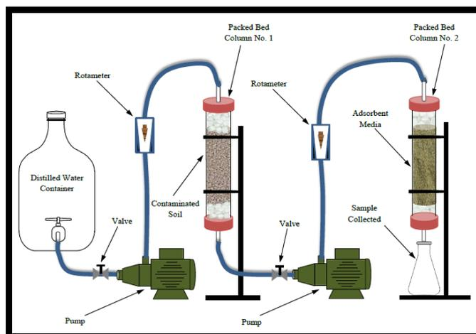
Figure 5: A schematic of continuous packed bed unit
