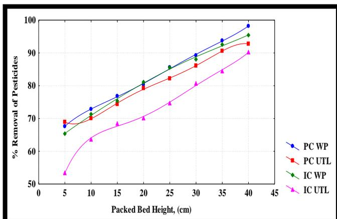
**Figure 10:** Influence of packed bed height on % removal of pesticides using residues. Where PC WP is pirimicarb removed by WP, PC UTL is pirimicarb removed by UTL, IC WP is imidacloprid removed by WP, and IC UTL is imidacloprid removed by UTL
