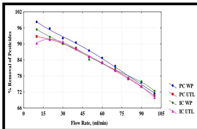
**Figure 11:** Influence of flow rate on % removal of pesticides using residues. Where PC WP is pirimicarb removed by WP, PC UTL is pirimicarb removed by UTL, IC WP is imidacloprid removed by WP, and IC UTL is imidacloprid removed by UTL
