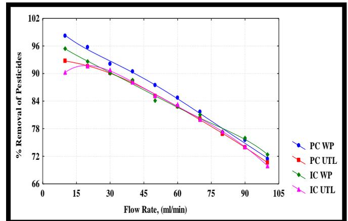
**Figure 11:** Influence of flow rate on % removal of pesticides using residues. Where PC WP is pirimicarb removed by WP, PC UTL is pirimicarb removed by UTL, IC WP is imidacloprid removed by WP, and IC UTL is imidacloprid removed by UTL
