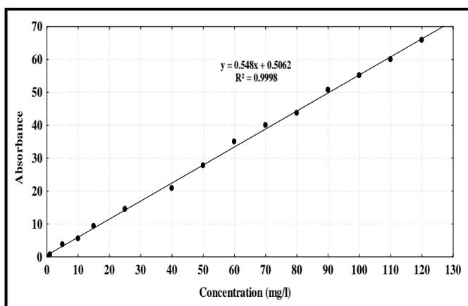
Figure 1: Pirimicarb pesticide calibration curve
