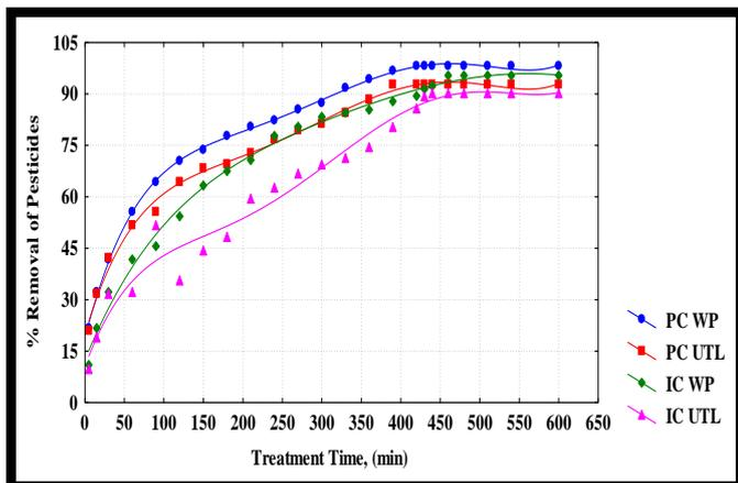
**Figure 12:** Influence of treatment time on % removal of pesticides using residues. Where PC WP is pirimicarb removed by WP, PC UTL is pirimicarb removed by UTL, IC WP is imidacloprid removed by WP, and IC UTL is imidacloprid removed by UTL
